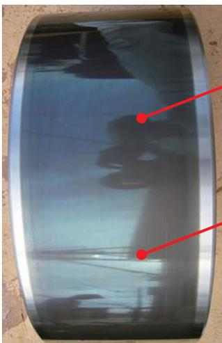
Confirm no cracking or chipping
