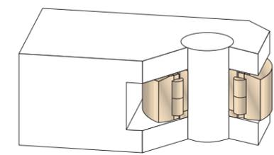
Cylindrical roller bearings for work roll thrust
