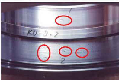
Brinelling on raceway surface of outer ring
