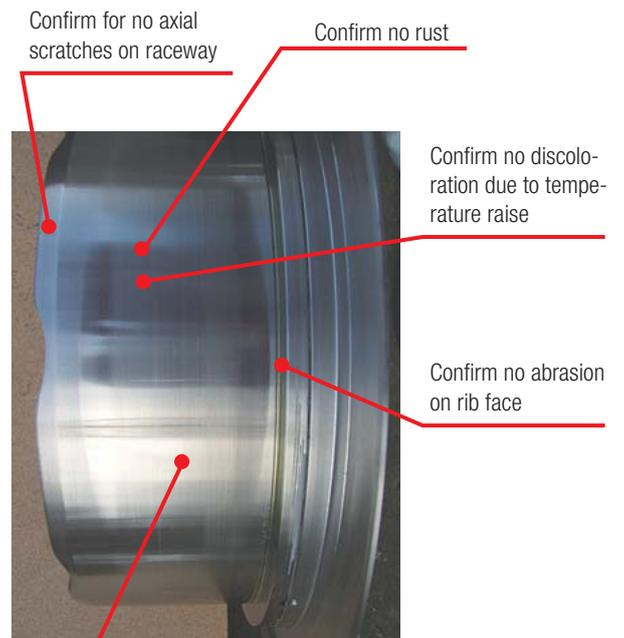
Confirm that race way has no unbalanced, asymmetrical roller contact marks on both rows.
