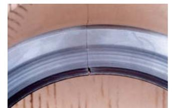
Inner ring cracking
