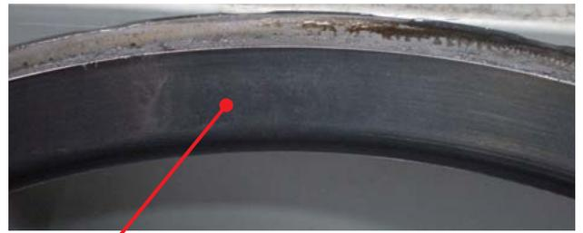
Confirm no cracking or chipping on seal lip part
