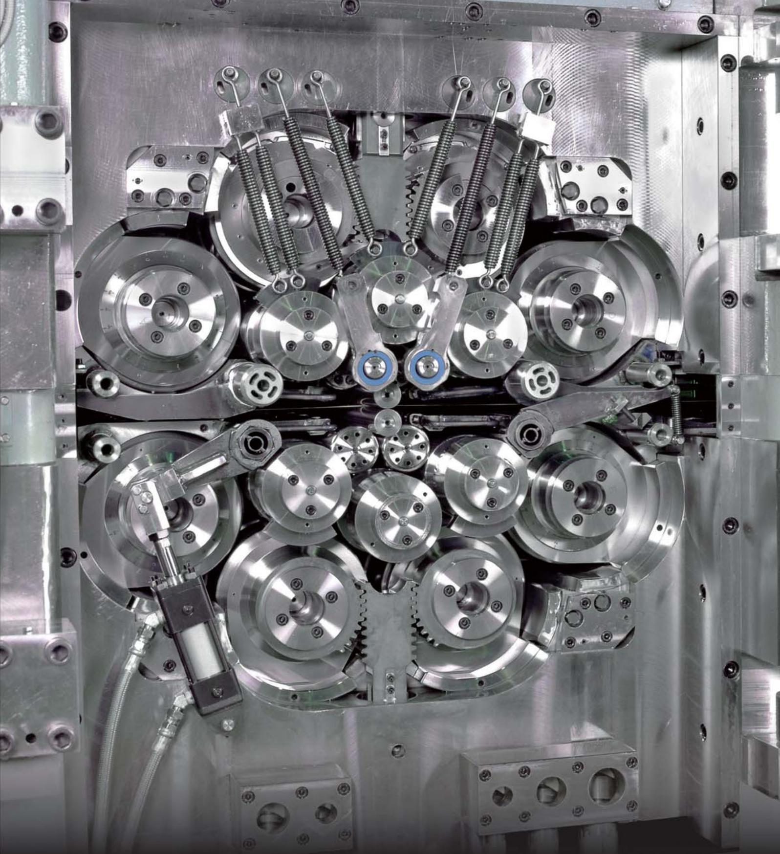
**Multi-roll mills enable our customers to utilize extremely small diameter work rolls with a choice of 12 or 20 rolls. Thereby, we are now capable of rolling hard materials such as stainless steel sheets and electrical steel sheets as well as rolling ultrathin copper. Cylindrical roller bearings for backup rolls play a significant role in obtaining this high level of efficiency.**
