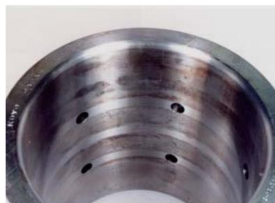
Fretting on bore surface of inner ring
