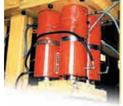
Four special order 500 ton, 24" stroke cylinders used in a swaging press for crimping 3 1/2" wire rope.
