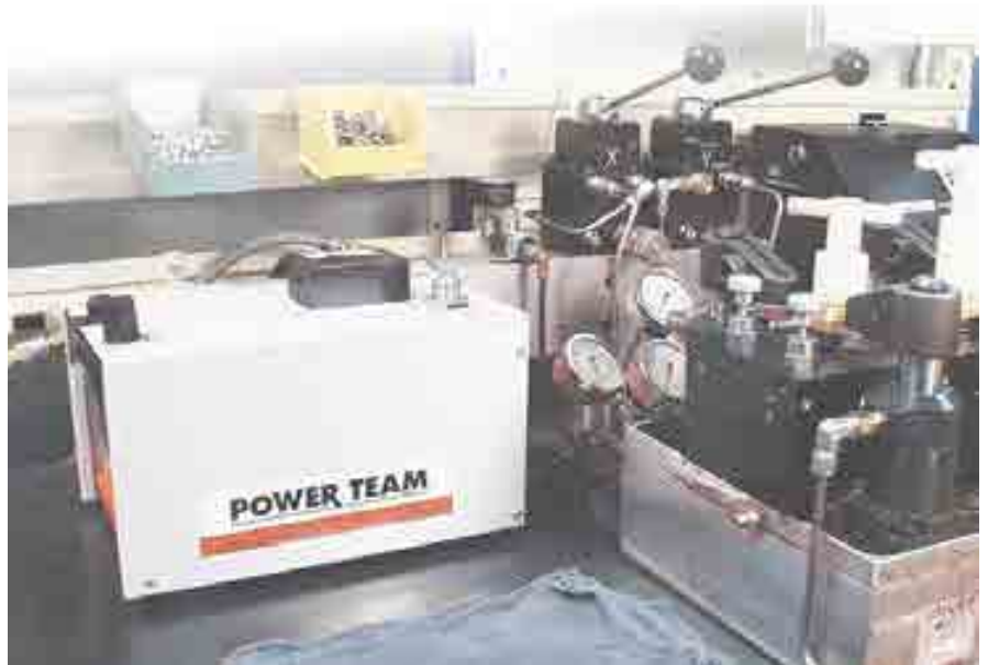
The PA60 used in a workholding environment.
